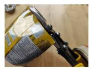
c. Fold this section over, encasing the sharp edges (left). Needle nose pliers can help with the folding (right).
