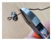
c. Wrap the other end of the wire around one side of your round nosed pliers to form the second loop.
