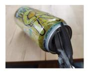
b. Cut out the side flat part of the pop can into square or rectangular sections.
