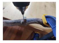
a. Mark how deep to drill your hole by comparing your drill bit to the eyehook you are using. Mark the drill bit with masking tape.
