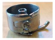
d. Machines with a removable bobbin case also have a removable assembly around it. This sometimes needs removing for cleaning out lint and freeing thread snags.
