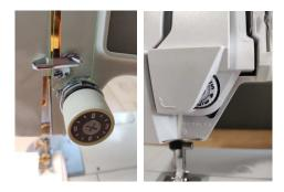
a. Some machines when threading you need to slip the top thread between the tension disks when threading the machine. This will be just above where the needle is.
