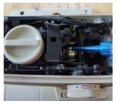
26. A small brush is useful for cleaning lint and debris out of your machine, particularly around the needle and bobbin case areas where it accumulates most.
