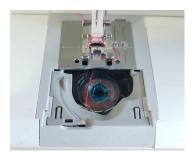
b. Some machines have a bobbin case with a tab you pull out the remove the bobbin case. It is accessed by a door that comes down at the front under the needle.
