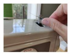
d. Run your top thread from the spool pin through the thread guide and insert the end into the hole on one of the edges of your bobbin or wrap it around your bobbin a few times. Your machine manual will specify which way around to wrap it to match the winding direction. Two styles are shown below.
