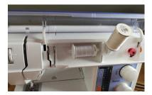
7. Sewing machines have a thread tension dial for the needle thread. This is adjusted based on the type of fabric you are working on. Tighter tension is general needed for thicker fabrics to pull the thread through. It is best to test the fabric and number of layers you are working with first.
