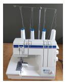
a. Overlockers also have a cutting blade that trims the edge of your fabric to the right width for edge finishing as you go.
