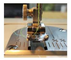
a. On some machines the feed dogs can be covered or lowered (right) by a button/switch (left) when you want to guide the fabric yourself, like during free motion embroidery. Some machines have a dial with a setting like # (centre) for lowering the feed.
