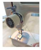
8. The presser foot engages the thread tension and holds the fabric down while sewing. Always lower the presser foot (centre) before sewing and raise it to draw thread through after (right). There is usually a lever behind the needle for raising and lowering (left).
