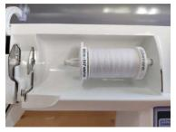
a. If there is a second pin then your sewing machine can likely take a twin needle, so two top threads. Sometimes the second pin comes as an attachment to add only when needed.
