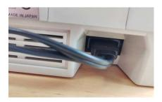
4. The control foot goes on the floor under your table and activates machine stitching or bobbin winding when the machine is turned on. With the presser foot down, press on the control foot gently to start sewing. The narrower edge is towards your heel. Pressing harder makes the machine go faster.
