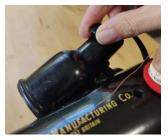
3. The control foot and power cord connect to the base of the machine. When attaching the cords be careful to push the cord attachment all the way in for the machine to work.
