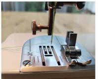
11. The sole plate is the metal plate directly underneath the presser foot with measurement markings.
