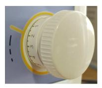
19. There is also a dial or method of setting the stitch width if your machine can do a zigzag stitch where the needle moves one side to the other for each stitch.
