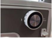
20. Sewing in reverse is useful to go back and forth on your stitching to anchor the start and end of a seam. There can be a setting, lever that stays in place or a switch you hold down while sewing in reverse.
