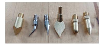
5. The tips unscrew from the end of the burning tool. Unplug your burning tool and allow it to cool before changing the point. Solid point tips are generally made of brass, which is a soft metal. Changing tips when it is hot can strip the screw thread. Many places recommend using pliers to screw points into the end of the burner pen. This can mark the brass tips so I prefer to change tips by hand when the tool is fully cool.
