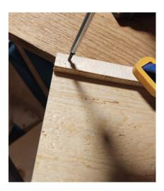
b. Attach the other narrow length of plywood at the bottom edge of your wood base, but on the other side.
